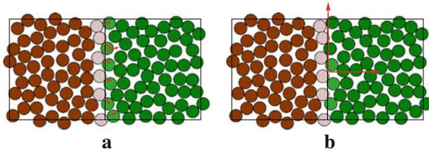
**Fig. 1** **a** A sketch of two neighbouring volume elements of the fluid share a layer surface, across which grains belonging to the different elements are in contact and transmit inter-granular forces; **b** The transmit inter-granular forces are coarse-grained into a normal and tangential force between the volume elements
